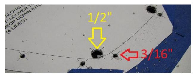
**2.17.** Using the template as a guide, cut out the section marked "cut out". The hood is steel and the paint is very easily burnt! This is normal and will be covered up with the flange of our hood louver.
