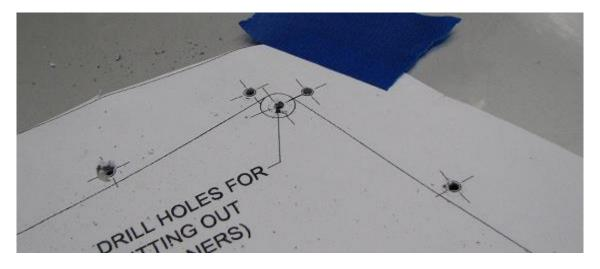
**2.16.** Enlarge the inside holes to  $^{\sim}1/2$ ". Enlarge the mounting holes to 3/16" initially.
