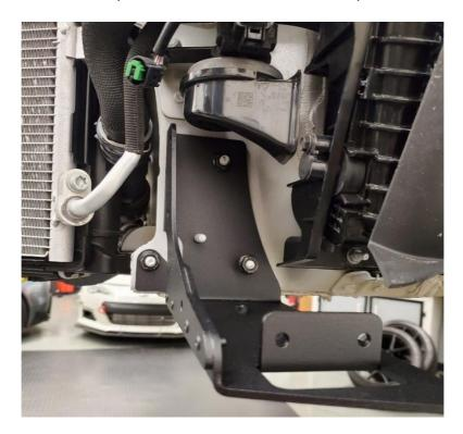
**2.16.** Using three 16mm long M6 BHCS, 18mm washers, and M6 serrated flange nuts, bolt the side splitter brackets to the main splitter brackets. Torque the bolts to 6 ft-lbs.
