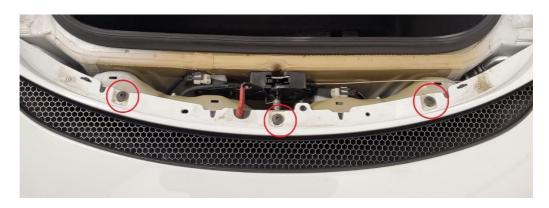
**2.10.** Using a small hook completely pull out the bumper release tabs on the inside of the headlight housing.
