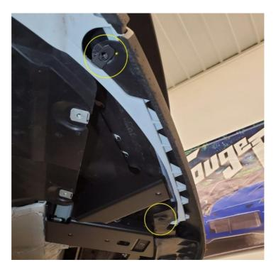
**2.24.** Next, transfer a U-nut from the previously removed center splash guard from **2.4** to both wheel liners.
