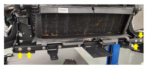
**2.18.** Next, assemble the three Cross Brace Brackets as shown. The two narrower brackets should be on the outside with the larger bracket in the center. Again, use 40mm long M6 BHCS, 18mm washers, and M6 serrated flange nuts. Torque to 6 ft-lbs.
