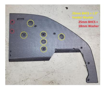
2.26. Install 30mm long M6 BHCS, 18mm washer, and spacers into the locations shown below
