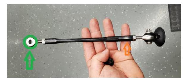
**2.20.** Reusing the 13mm nut from the tension cable, bolt the support rod to the crash bar, and use a 12mm M6 BHCS with 12mm washer to bolt the clevis to the cross brace. Torque the M6 BHCS to 6 ft-lbs, and the OEM 13mm nut to 13 ft-lbs. The support rod should be passing through the radiator duct cut-outs as shown below.
