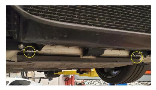
**2.26.** Bolt the side chassis brackets to the main splitter brackets with 20mm long M6 button head cap screws, and 12mm O.D. washers. Torque to 6 ft-lbs.
