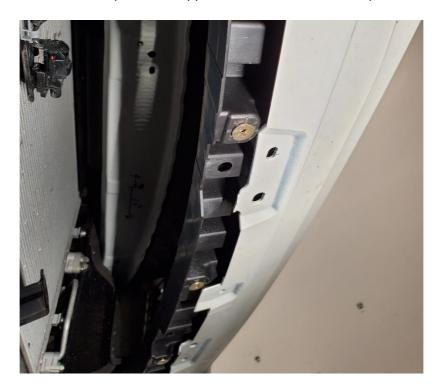
**2.14.** To install the splitter rods we will need to measure the point to drill for rivet nut installation. Looking upward at the crash bar, locate the two slotted holes.
