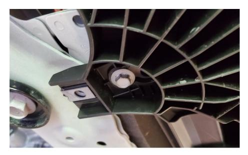
**2.24.** Next, we will begin putting the splitter up using seven 40mm BHCS, fender washers, and 5mm spacers in the holes shown below. Starting in the middle, and working your way outward is the easiest way to get this done. Do not tighten the bolts down at this time.
