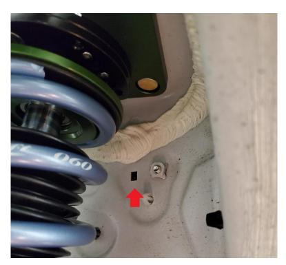
**2.11.** Install the 10 mm long M4x.7 BHCS, and fender washer into the threaded hole. Torque to 3 ft-lbs.
