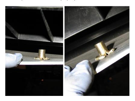
**2.14.** Once the front and rear rivet nuts are installed, temporarily bolt the side splitter to the car using 25mm BHCS, fender washer, and 18mm O.D. washer. The 18mm O.D. washer should be used for the front bolt. Bottom the bolts out so that the side splitter sits flush up against the side skirt.
