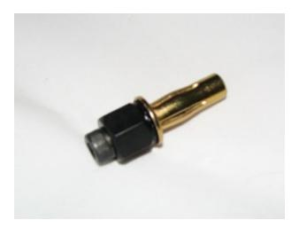
**2.11.** Using the 9/16" wrench and the 5mm allen wrench, hold the nut steady and tighten the allen bolt. You will have some initial resistance, then the rivet nut will begin to pull tighter on the material.
