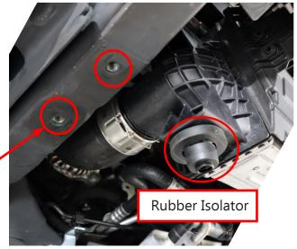
Install the new Intercooler Mounting Bracket by reusing the stock Recovery Bracket mounting bolts.
