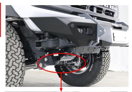
You will need the two black bolts that were used to hold your stock front air dam or skid plate located here.
