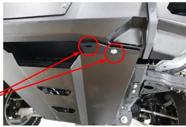
Install the Ø3/8" Button Head Screws, Washers and Nuts onto the Lower Front Skid Mount. Once all fasteners are installed, be sure to tighten every one securely.
