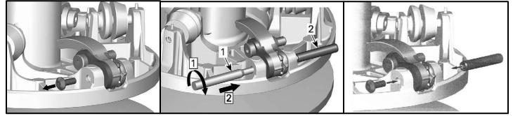
Unscrew the Bolt that holds the clutch weight in, then install the tool to remove the pin as it is pressed in. This will require some slight tapping to remove. After the clutch weigh is removed you can install the stock Skidoo components onto the Straightline clutch weight. The Explode view above will show proper assembly.
