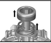
Remove spring cup, install spring after installation of clutch weights
