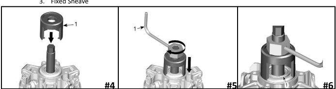
**Install Puller Stud Compress Spring Cup** Remove Circlip #1 Straightline Performance 15250 Hornsby St Forest Lake, MN 55025 651-466-0212 www.straightlineperformance.com
