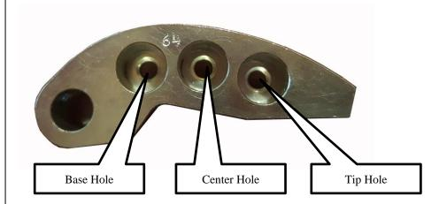
Remove the primary clutch and install the weights and primary spring. Remove secondary clutch and install new helix in proper setting, with spring. Inspect all internal clutch components for wear. If excesses wear is prevalent replace needed items.
