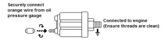
**Make sure** that the connection between the oil pressure sensor and the engine is clean and **does not** have Teflon tape or any other sealants on the threads. This provides a stable ground for the sensor which will not function if it is inhibited.
