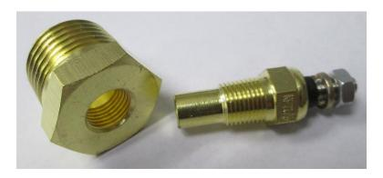
This sending unit may be used with our M9013 Water Temp Gauge; M9108 Oil Temp Gauge or M9107 Transmission Temp Gauge. It is supplied with an optional bushing. The wire from your selected gauge should be connected to the terminal at the top of the sender.
