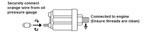
**Make sure** that the connection between the oil pressure sensor and the engine is clean and **does not** have Teflon tape or any other sealants on the threads. This provides a stable ground for the sensor and will not function if it is inhibited.
