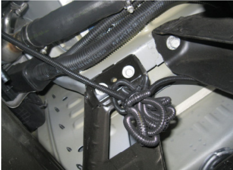
Figure 23. Excess wiring harness zip tied near the bed pass through grommet.
