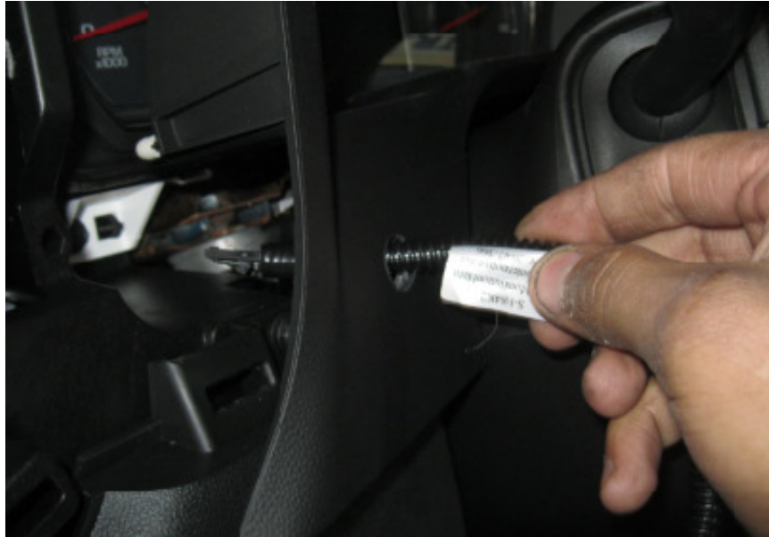
Figure 20. Manual pump operation button.
