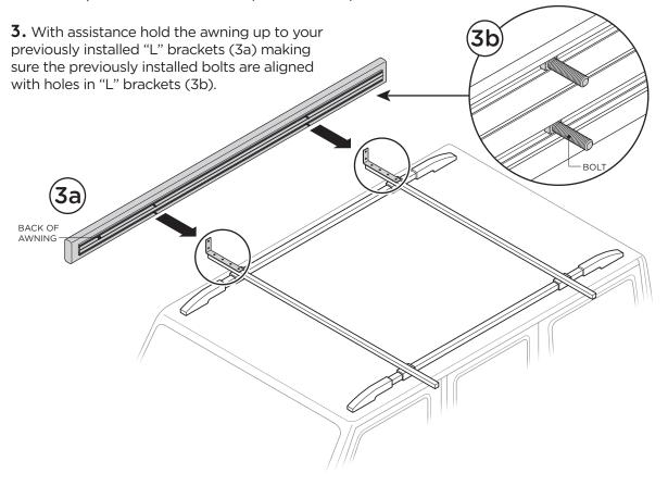
4. Secure each "L" bracket with bolts using two (2) washers and two (2) nuts per bracket (4a). Fully tighten (4b).
