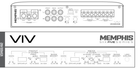
Controls are located under top plate for easy access
