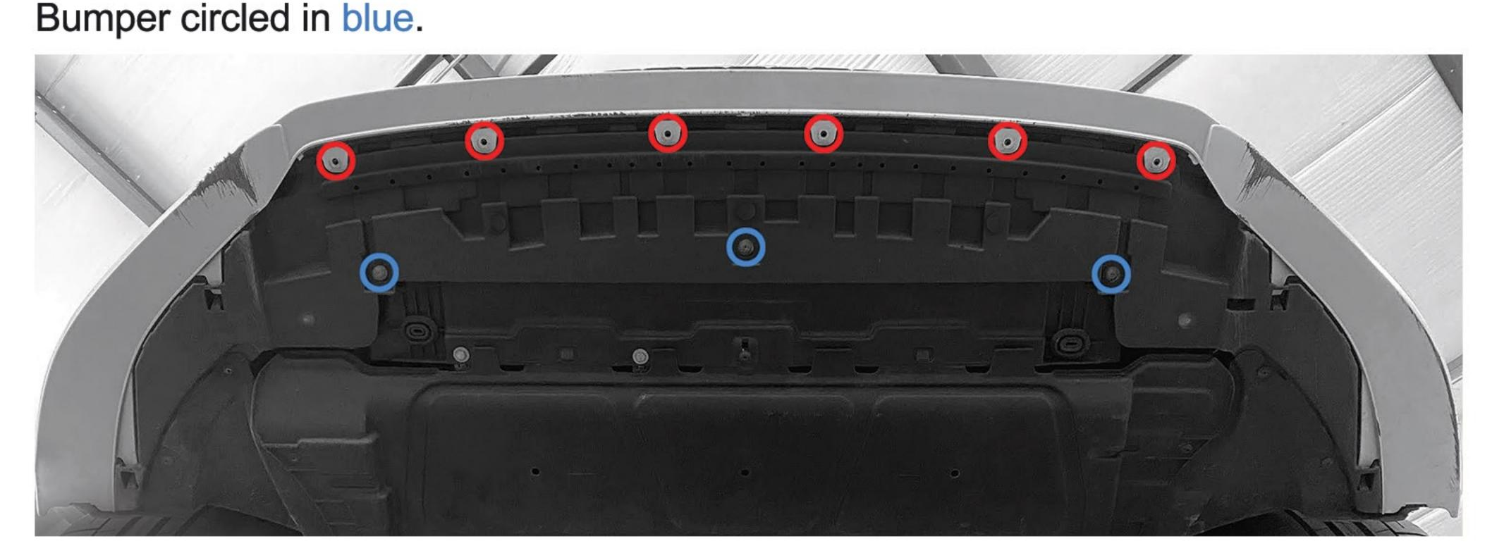
3. Place the aerofabb Splitter on underside of Bumper. Using a T-25 Torx, install 4 fasteners from HARDWARE (A) into Bumper holes (A). Using a T-30 Torx, install 2 fasteners from HARDWARE (B) into Bumper holes (B).
