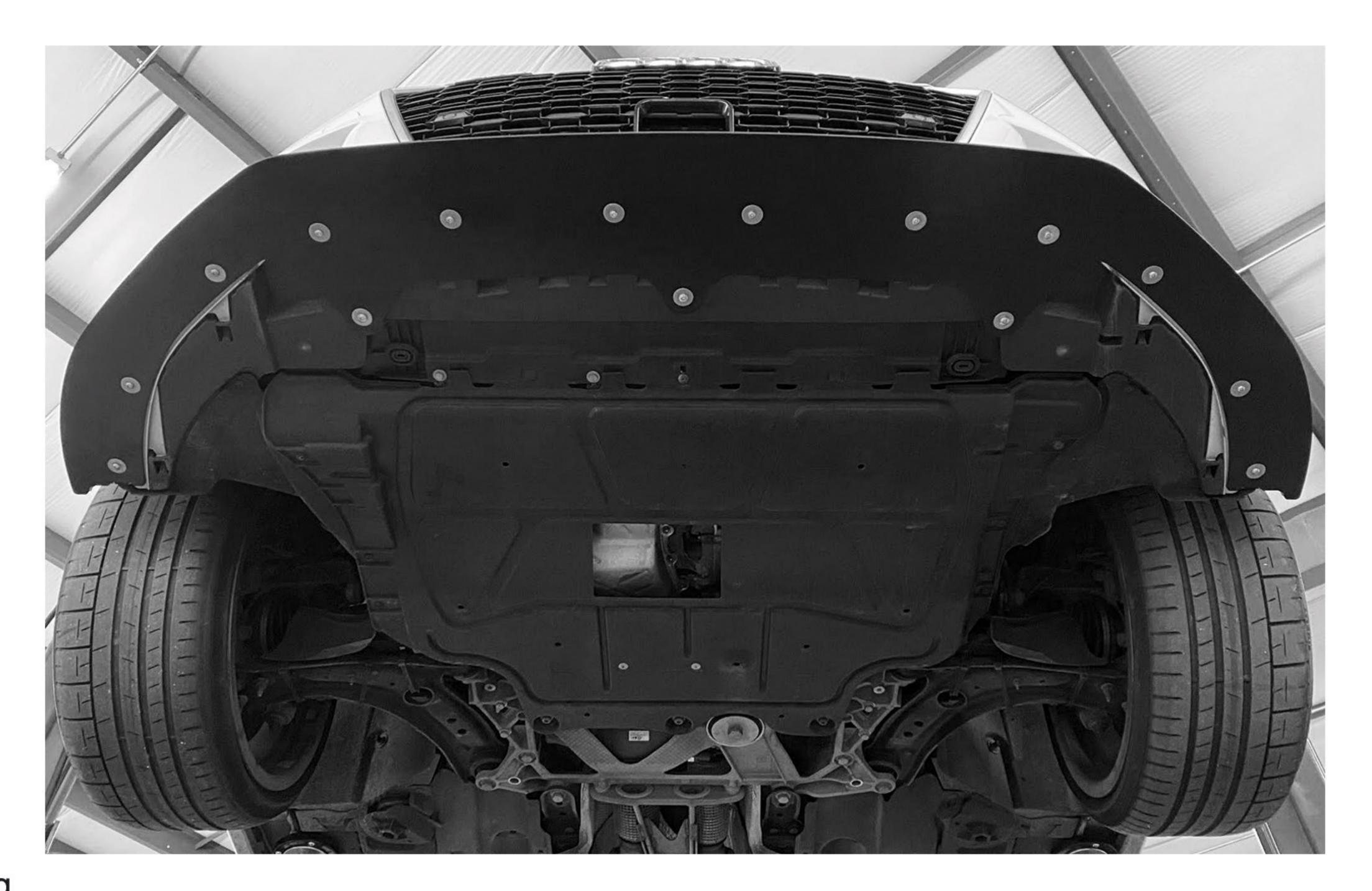
10. Inspect all hardware for tightness to complete Front Splitter installation.
