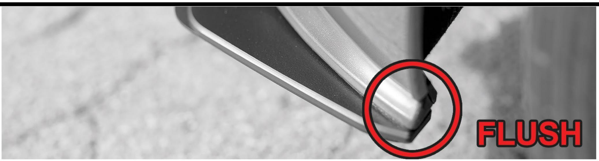
7. With the Side Spats aligned correctly, use a **Light Colored Marking Tool** to mark through the pre-drilled Spat holes (C) and onto bottom side of Factory Valance. With holes marked, remove **HARDWARE** (B) and Spats.
