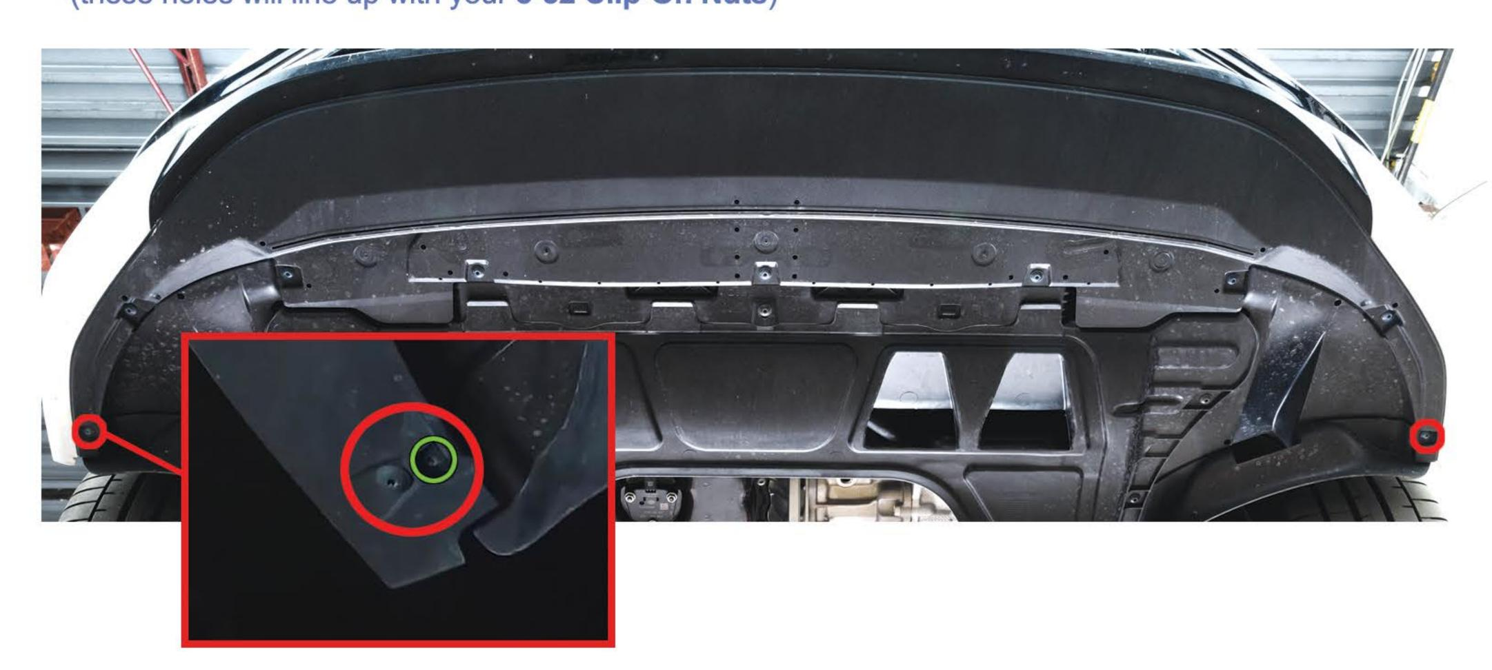
9. Using a **3/32**" **Hex Wrench**, install the remaining hardware from **ALIGNMENT HARDWARE (B).** Fasten Splitter to Bumper by passing through Splitter holes **(B)** and tighten.
