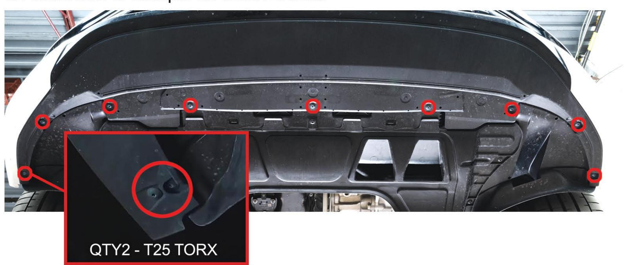
3. Using a **T-25 Torx**, identify and remove the 6 lower Fender Liner Torx screws. (3 in each Wheel Well on Bumper Side)
