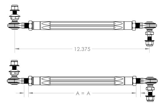
For cosmetic purposes, to avoid scratching the blue anodizing, we suggest using an aluminum adjustable wrench or applying masking tape to a normal wrench. The sleeve size is 3/4" and the jam nuts are 11/16".
