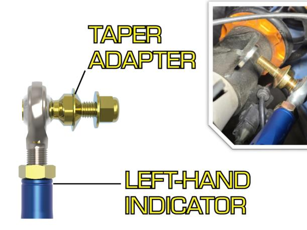
\*IMPORTANT: USE A TORQUE WRENCH AND TIGHTEN THE END LINK NUTS TO **35 FT · LBS**. <u>DO NOT USE AN IMPACT GUN ON THE END LINK NUTS</u>. OVERTORQUING THE NUTS CAN LEAD TO STUD FAILURE.
