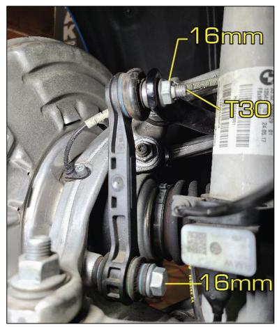
4R Set the aFe Control end link to 5.188" center to center. Make sure to have equal thread engagement for each rod end when adjusting.
