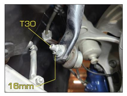
5F Set the aFe Control end link to 12.375" center to center. Make sure to have equal thread engagement for each rod end when adjusting.
