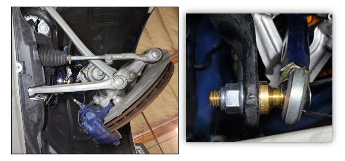
Rotate the entire end link **counterclockwise** while rotating the bottom rod end **clockwise**. Now, back off the bottom rod end from full clockwise and leaving about 20° of rod end play as a buffer. Tighten the jam nut. Rotate the end link back and forth to make sure there is still about 20° of rod end play.
