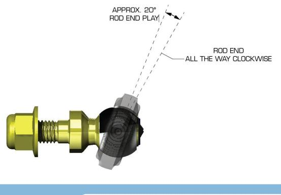
Next, turn the wheel all the way to the right and make sure the end link has the same amount of rod end play. This will ensure your rod ends will never run out of articulation when steering.
