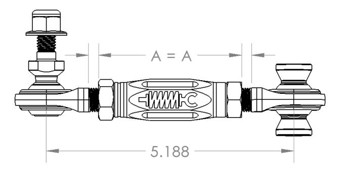
Optional: For cosmetic purposes, to avoid scratching the blue anodizing on the sleeve, we suggest using an aluminum adjustable wrench or applying masking tape to a normal wrench. The sleeve size is 3/4" and the jam nuts are 11/16".
