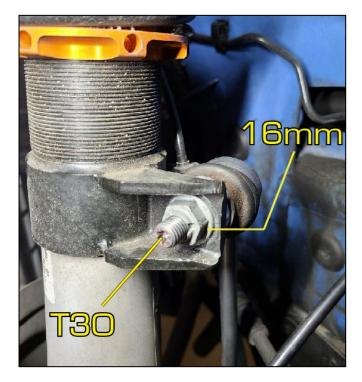
4F Unbolt the end link from the sway bar using a T30 socket and 16mm as well. Remove the factory end link from the car. Mark "left" on the end link for reference.
