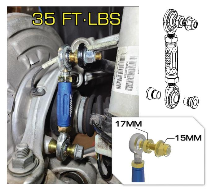
6R Repeat for the passenger side. Reinstall wheels and torque lug bolts to 105 ft · lbs.
