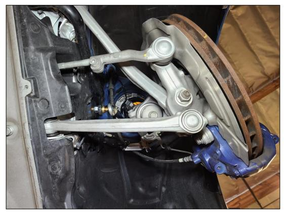
8F Repeat for the passenger side. Clocking and positioning will be a mirror image of the left. Reinstall wheels and torque lug bolts to 105 ft · lbs.
