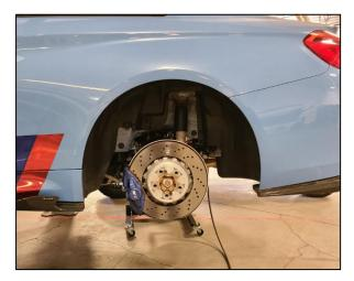
3R Unfasten the left end link from the car using a T30 socket to hold the stud and a 16mm wrench to undo the nut at the top. Use a 16mm socket or wrench for the lower bolt.
