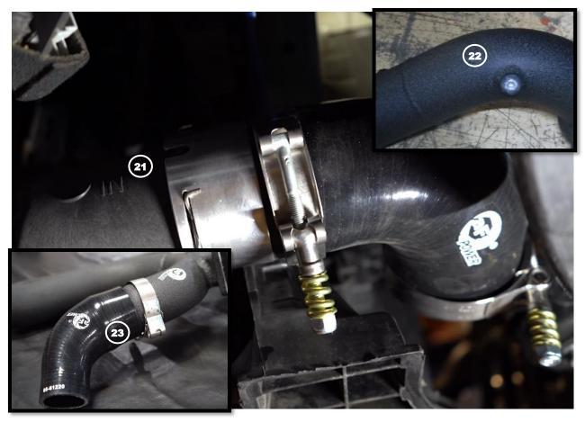
28. Install the aFe adaptor onto the intercooler and line the notch up with the intercooler 21
