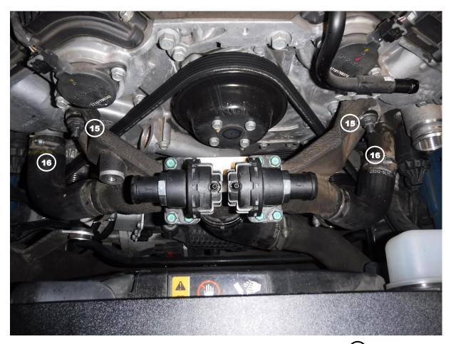
20. Remove the two nuts securing the hot side charge pipe to the engine 15
