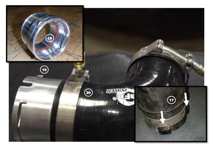
Note: The retaining clip will need to be removed from the factory charge pipe for reuse with the aFe charge pipe
