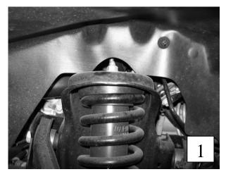
**2c**. Remove the bottom mounting bolt of the spring/strut assembly (**Photo 2**)
