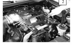
strut tower brace. Position the brace so that it does not touch the support bracket and so that the end brackets are flat against the strut tower and firewall. Keep the brace close to the air intake tube, going to the throttle, to prevent it from interfering with the hood.
