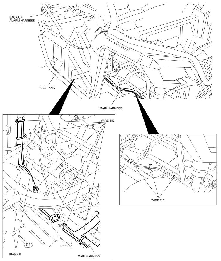
5. Follow the main harness going up. Secure the back up alarm harness to the main harness with wire ties along the front right side of the vehicle as shown.
