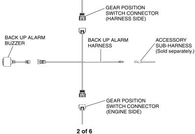
4. Follow the main harness down. Secure the back up alarm harness to the main harness with wire ties near the back of the engine, under the passenger seat as shown.
