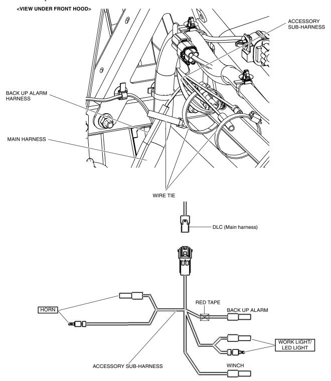
8. Install the back up alarm buzzer to the location shown:
