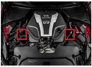
Red Boxes are where you should be able to fit socket with extension down to the top nuts.
