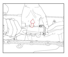
**IMPORTANT:** While the bolts are started, but still loose, lift the pickup tube. Tighten the two bolts while maintaining the lifted position. This process ensures proper clearance between the pickup inlet and the pan floor.
