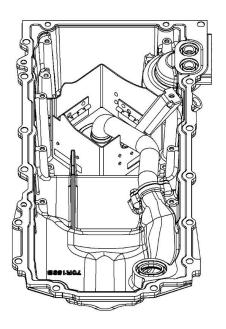
**IMPORTANT:** While the bolts are started, but still loose, lift the pickup tube. Tighten the two bolts while maintaining the lifted position. This process ensures proper clearance between the pickup inlet and the pan floor.
