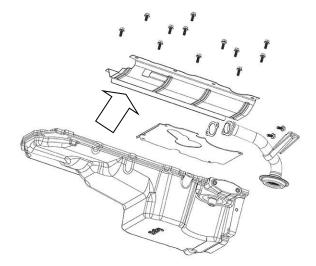
IMPORTANT: All gasket surfaces should be free of oil or other foreign material during assembly. Inspect the engine block
