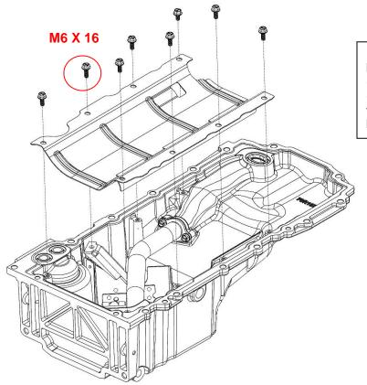
Reinstall the windage tray. Apply a drop of blue Loctite® to the threads of the supplied (x7) M6 x 12 flange head bolts. Install the (x1) M6 x 16 flange head bolt in the location that also goes through the pickup tube bracket. Torque the bolts to 10 lb./ft.
