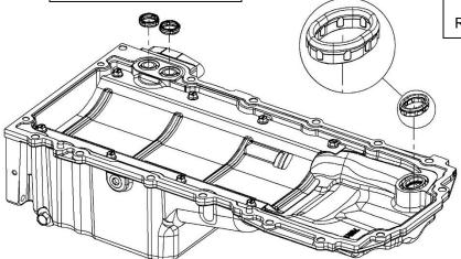
Confirm pickup to oil pump seal is still in place. **WARNING:** This seal must be oriented as pictured.
