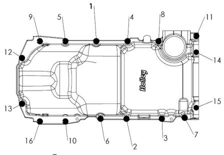
Torque: M8 bolts to 18 lb./feet. (bolts 1 through 13). M6 bolts to 106 lb./inch. (bolts 14 and 15).
