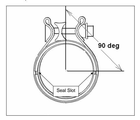
8. Make sure the tailpipes and tips are aligned and have clearance to the rear fascia. Torque both band clamps to 35 ft-lbs.
