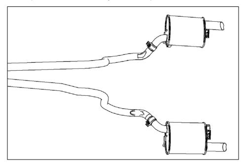
2. Loosen both ends of the doubled-sided clamps, which hold the midpipes in place. These clamps are located after the H-pipe.
