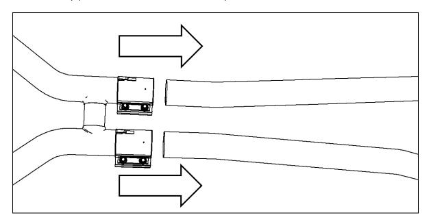
4. Slide both midpipes out of the muffler flanges and remove both midpipes from the vehicle.
