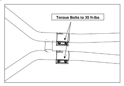
6. Slide the band clamps into position over the tailpipe and midpipe connection points. Make sure the clamp band covers the seal slot, as shown below. This will prevent exhaust leaks.
