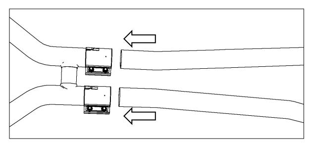
4. Install each midpipe into the flared end of each tailpipe. Make sure the midpipe is fully seated into the tailpipe flange.
