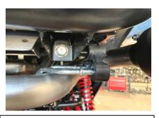
4. To install the Gibson muffler (Item A), re-install the factory rubber insulators on your new muffler assembly and install the muffler onto the factory hangers. Then install and tighten the flange bolts for the head pipe using Item G) included in the kit are shorter flange springs.
