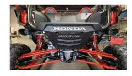
**6.** Finally, slide each tip(Item D) onto each tail pipe up to the rivets and secure using the included bolt kit.
