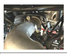
2. Remove the two factory bolts with springs from the headpipe and set aside to re-use later. Do not damage the factory exhaust gasket. You will re-use this gasket. Then loosen the O2 sensor and lay it aside for later re-installation.
