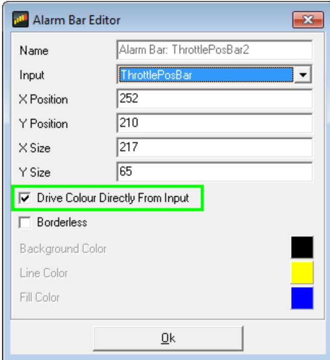
Set the input to the appropriate channel and check Drive Color Directly From Input. All other Alarm Bar functions beyond this are the same as previous versions.
