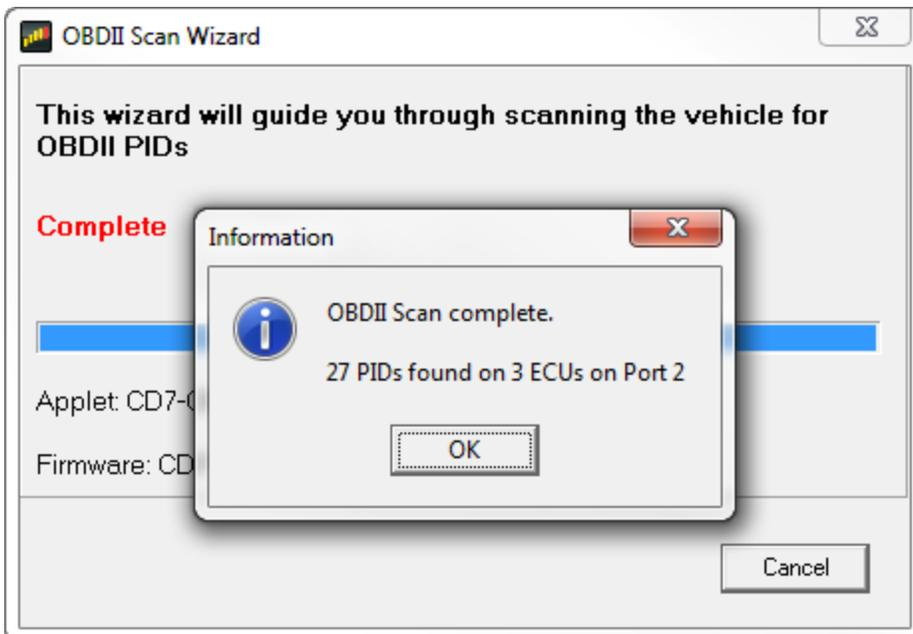
The scan is complete. Click OK to proceed. **NOTE: At this point, we recommend saving the setup file as there may have been changes applied during the scan process. You must upload your setup before proceeding by selecting File | Upload to Display... You can also use the hotkey combination Ctrl+U. If the setup file is not loaded into dash after completing OBDII Scan Wizard there can be errors or missing data.**
