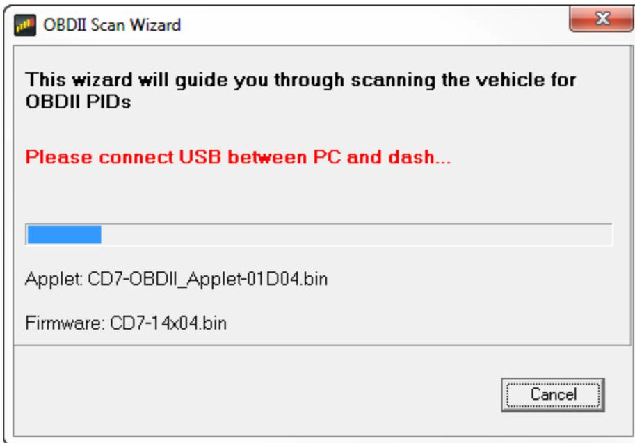
Be sure the dash is powered up and connect the USB cable between the dash and your PC and not plugged into the car yet.
