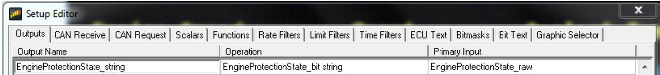
The next example uses EngineProtectionState\_raw as the Primary Input. This input has two possible values with are 0 or 1. A Bit text operation is used to convert these values into text texts that can be displayed on the dash.
