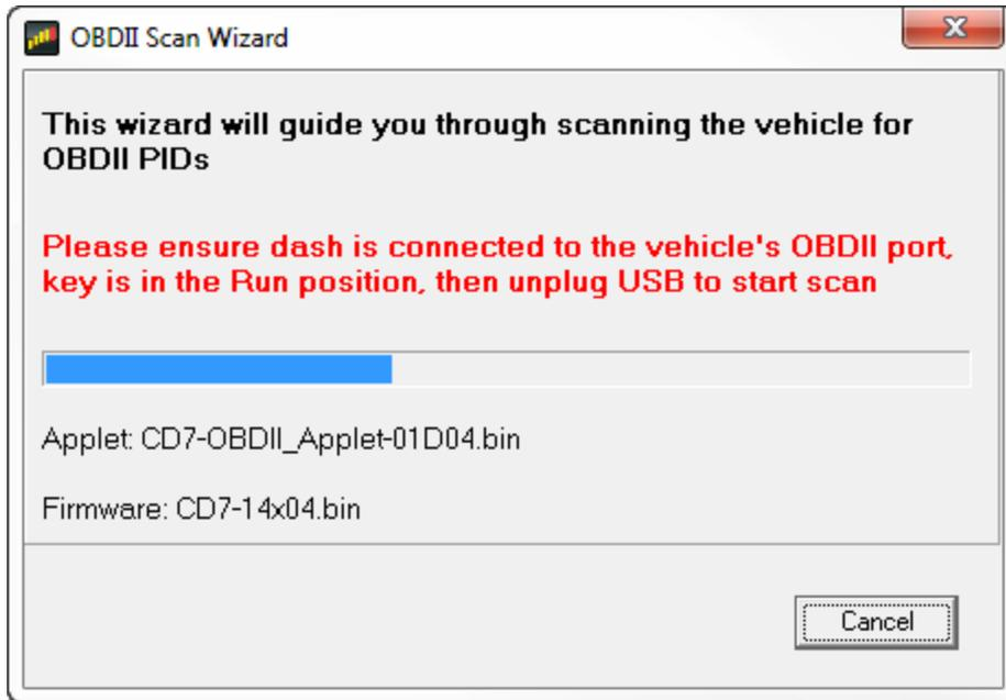
Connect the OBDII connector to your vehicle's OBDII port then unplug the USB cable to begin the scan.
