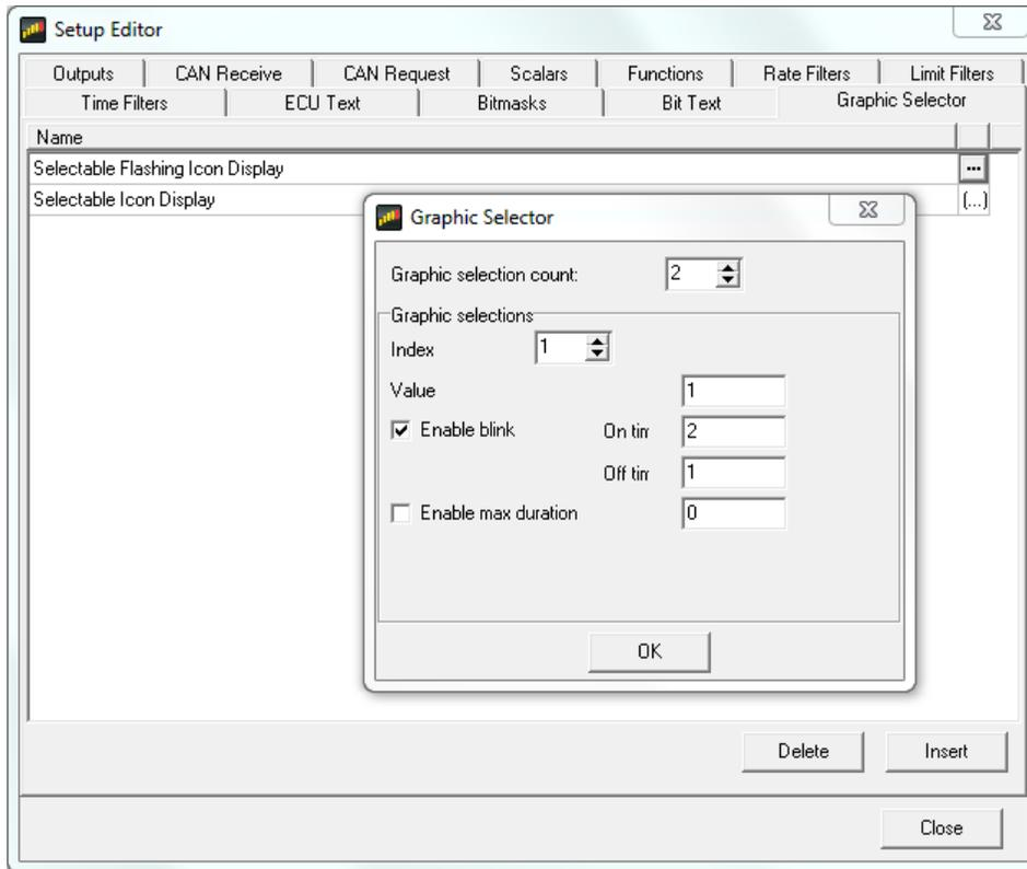
The graphic selection count is the number of graphics used in the sensor and is at least two. The first graphic is shown by default. Subsequent graphics are shown according to the settings in the graphic Selections box.
