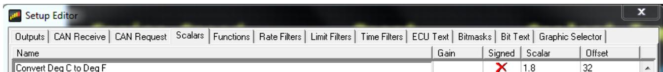
This Scalar operation uses a Scalar value of 1.8 and an offset value of 32. Applying this Operation results in the following math expression.
