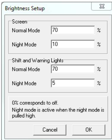
The Brightness setup dialog allows you to choose two different brightness settings for both the screen and LEDs. See [Harness and Wiring](#) section for Night Mode input wiring. 100% should only be used in direct sunlight. 70% gives almost as much brightness without overdriving the backlight. 5%-10% is appropriate for night mode. **NOTE: The LEDs used in the CD-5 unit are brighter and may require different settings compared to a CD-7 unit.**
