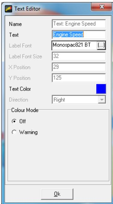
The dialog allows editing of all unlocked characteristics if Layout Locked is turned on. Locked characteristics are typically related to size and position. To change the text displayed in the text label example above, simply highlight the text and edit. Double clicking on the "0" in the example above opens the value label editor. This is live data displayed on the screen.
