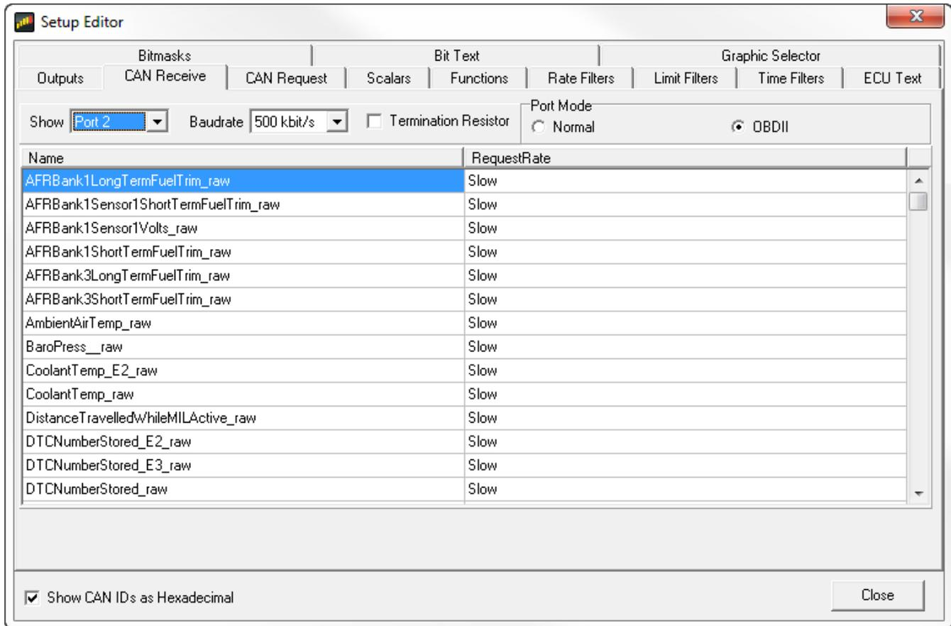
This is a complete listing of available PIDs. An AEM supplied setup file for OBDII messages will be located in the \Documents\AEM\DashDesign\Setups\Generic folder. The basic default OBDII file is named Default-Black-OB2.aemcd7.
