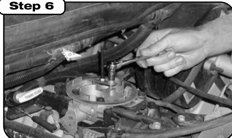
Install throttle body cap hold down bracket assembly.
