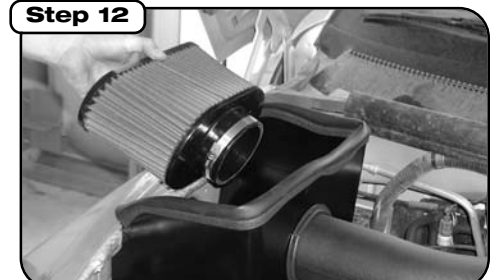
Attach filter to intake tube. It may be a tight fit, but DO NOT OIL OR GREASE TO INSTALL.
