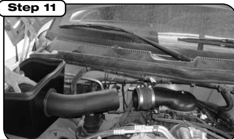
Insert tube through filter housing and attach to coupler with supplied clamps.
