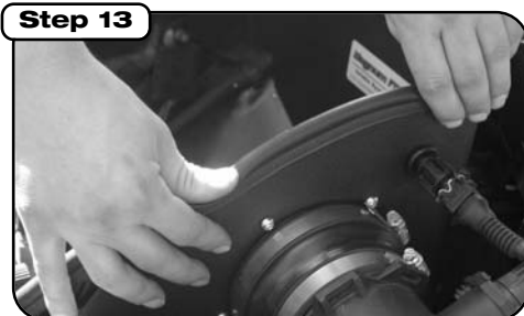
Install trim seal.
