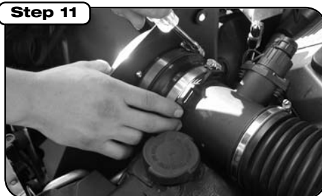
Tighten down 2 clamps that are used on the rubber adapter.
