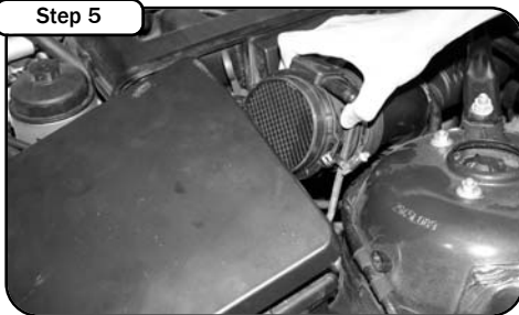
Step 5 Remove MAF sensor from airbox. Make sure you do not damage the rubber gasket. Lift airbox out and remove from vehicle.
