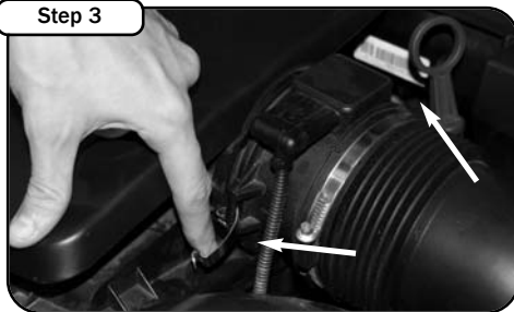
Step 3 Disconnect negative terminal from battery. Loosen the hose clamp on the intake tube. Disconnect the two metal clips on the side of the MAF sensor.
