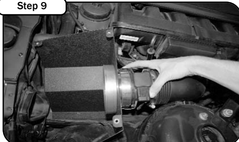
Step 9 Lower housing into the engine bay. Fasten the MAF sensor to the housing and secure with the two spring clips.
