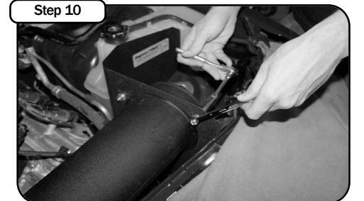
Align the mounting holes on the tube and the housing. Secure the assembly with the provided M6 bolts washers and nuts.
