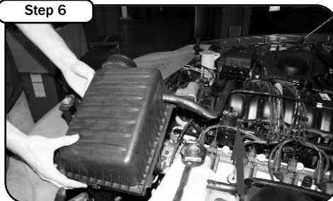
Remove the 5/8" breather hose on the side of the valve cover. Remove airbox assembly out of the engine bay.
