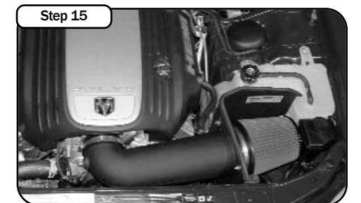
Your installation is now complete. Tighten all connections and clamps. Re-check after a few hours.
