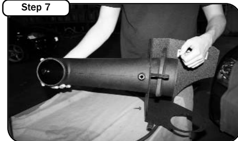
Slide the intake duct into the housing make sure you line up the mounting holes correctly.
