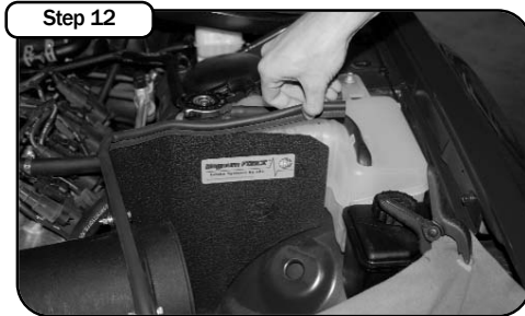
Install trim seal along the edge of the housing. Start at one end and work your way around the housing.
