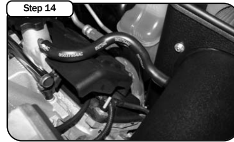
On SRT-8 models re-use factory crank case breather hose (shown in above photo). On non SRT-8 models use provided hose and clamps.
