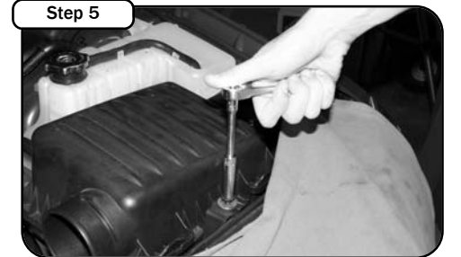
Remove the 10mm screw securing the airbox to the vehicle. Save for re-use later.
