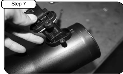
With provided T20 torx bit loosen the 2 bolts that hold in the MAF sensor. Carefully remove MAF sensor out.
