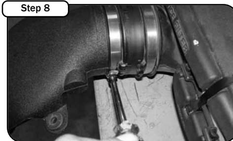
Step 8 Loosen the clamps holding the OE intake tube to the OE air box. Remove the tube.
