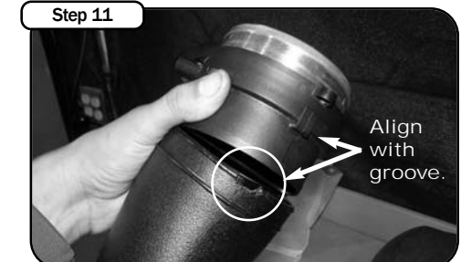
Step 11 Insert the MAF sensor into the aFe intake tube. Make sure to align the MAF sensor to the groove on the intake tube. This assembly requires a snug fit. If fit is too tight the tube can be heated with a hair dryer or heat gun to allow insertion.
