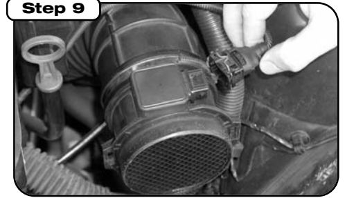
Install mass air flow sensor, tighten clamp with 1/4" nut driver and connect mass flow sensor plug.
