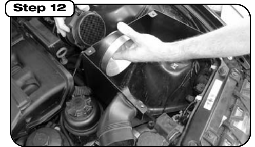
Install shield into vehicle, attach snorkel, and slip on mass flow sensor and attach spring clips.
