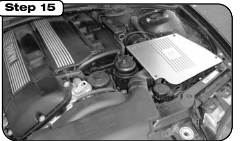
Place enclosed CARB EO sticker on a clean/smooth surface on or near the intake system. EO identification label is required in passing the Smog Check inspection. Make sure all hoses and clamps are tight and that all electrical components are secure.
