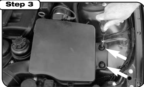
Remove two screws with 10 mm socket or wrench.
