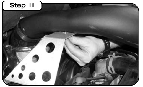
Line up the mounting holes on the intake duct and tighten assembly with the provided screws and washers.
