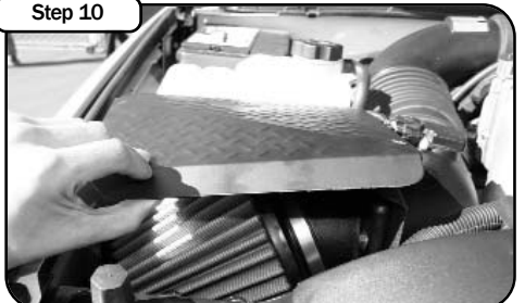
Reconnect the MAF sensor harness. With 3 button head screws, install the housing cover. Tighten with allen wrench.
