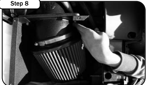
Install stage 1 tube outside of the housing and tighten all screws with 7/16 and 3/8 wrench or socket.
