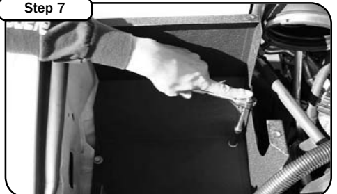
With 10mm wrench or socket, make sure to remove the factory airbox mounting plate bracket. With airbox bracket completely out, Lower new aFe housing in place. Use factory 10mm screws to secure the housing. Tighten all four screws.
