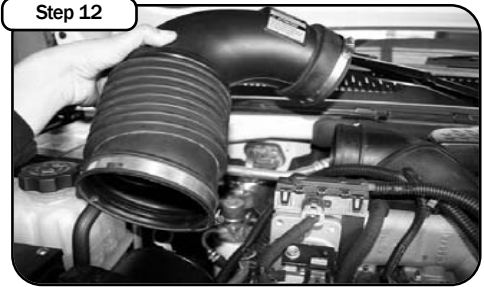
Additional steps for Stage 2 & Torque Booster Tube installation: With 5/16 nut driver loosen both clamps on factory tube and remove.
