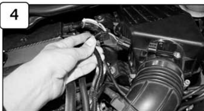
Disconnect MAF sensor harness.
