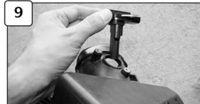
Remove MAF sensor from stock air box using phillips screwdriver.
