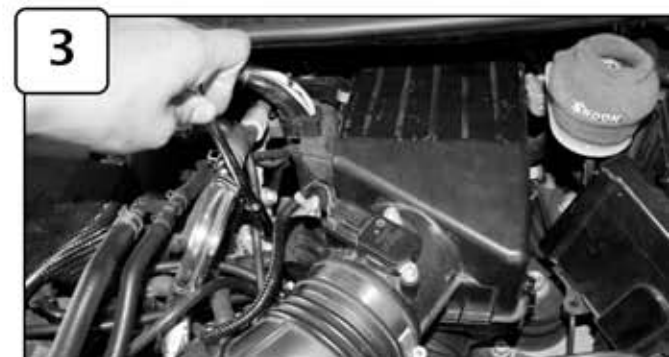
With 10mm socket or wrench, loosen the 2 bolts securing the stock air box.
