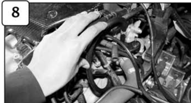
Replace throttle body coolant line with 5/16" hose provided and secure with clamps used from step 7.
