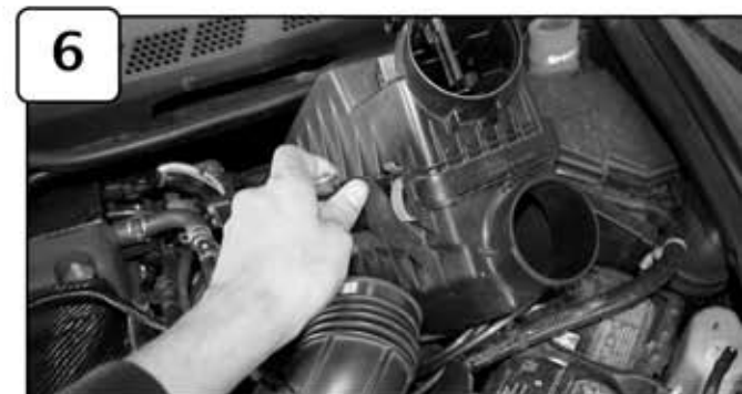
Remove complete stock air box out of vehicle including intake tube.
