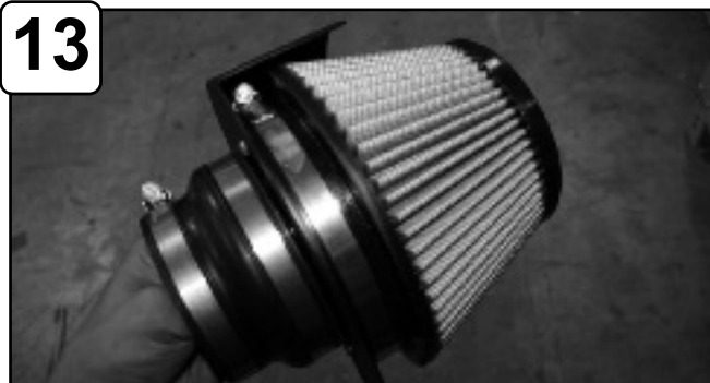
13 Install air filter and tighten using 5/16" nut driver. Attach 05-00612 coupling with clamps to adaptor and tighten. Attach rubber trim to side of housing to prevent contact with battery.
