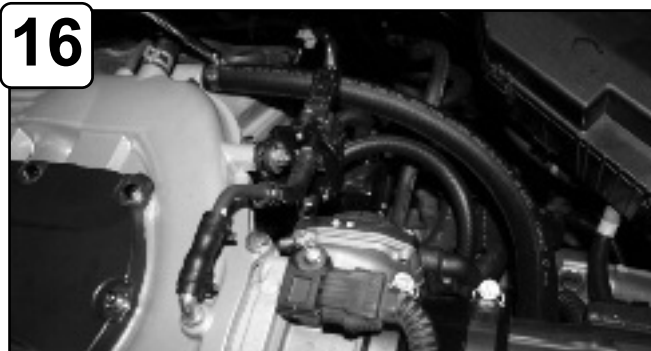
16 Install provided 5/8" hose to tube and engine. Using provided clamp tighten on engine side only.
