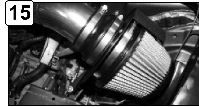
15 Install housing into vehicle and position tab to isolation mount from step 11. Note: Tube may need to be positioned to fit cut out on factory engine cover.
