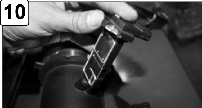
10 Remove MAF sensor from stock air box. Install into new tube and secure using provided M4 screws.
