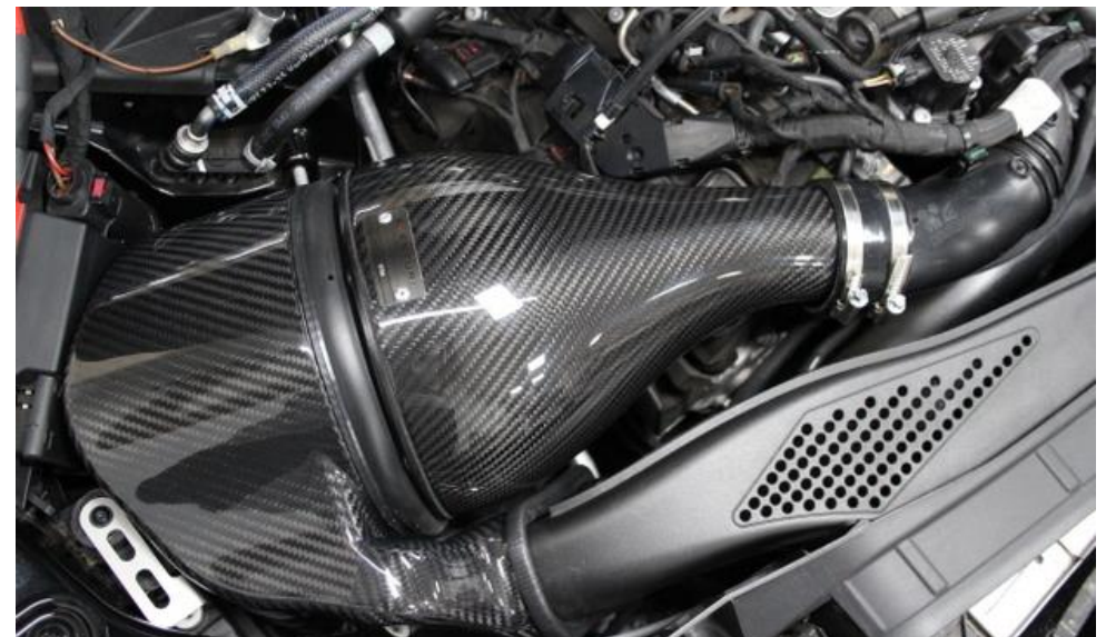
20. Carefully push the housing down into position – rotate the housing so that the bracket lines up as shown in the next step.
