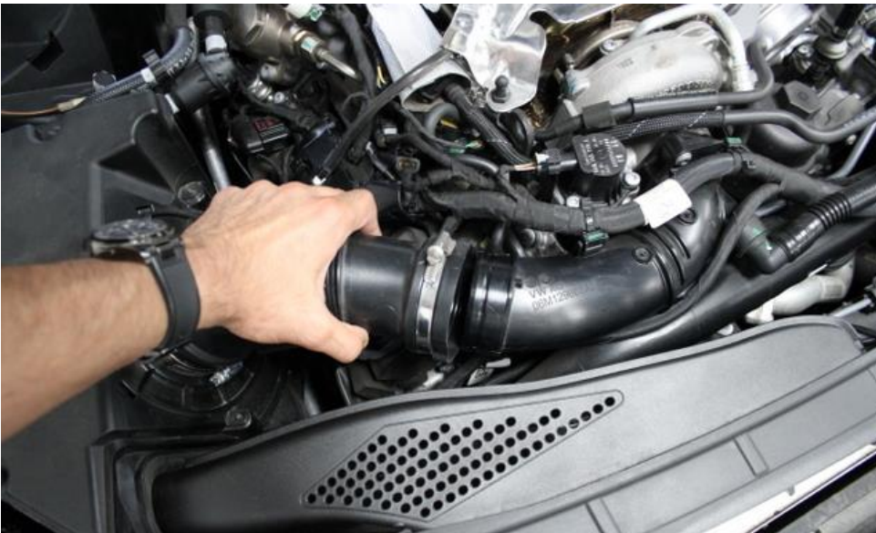
7. Loosen hose clamp connecting the airbox to the turbo inlet tube and pull the airbox away from the tube.
