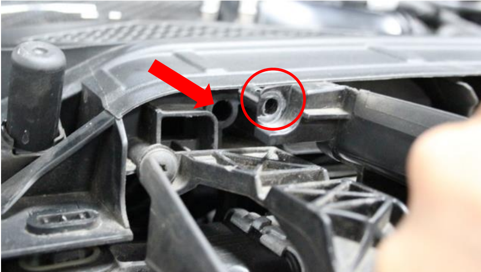
29. Relocate the front duct trim into its original position – the boss for the torx screw should go into the hole in the slam panel.
