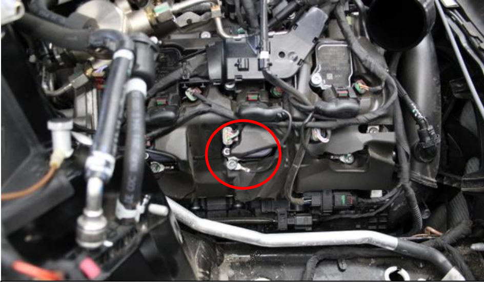
13. The filter housing will secure to the side of the engine. Remove the torx screw shown here – next photo shows a close-up.
