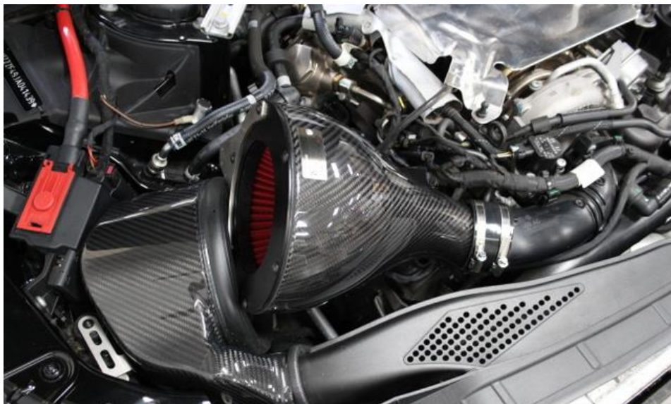
19. Position the filter housing so the Eventuri badge is facing upwards – push the outlet into the silicon coupler as shown.
