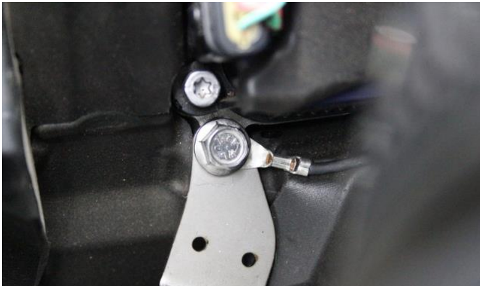
23. Secure the bracket using the supplied bolt – make sure the earth wire is also re-positioned and secured.
