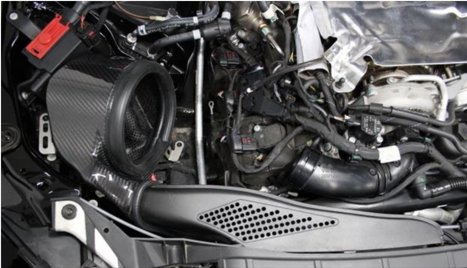
17. Push the stock duct trim into the carbon duct and position into place – do not secure with the screws yet.
