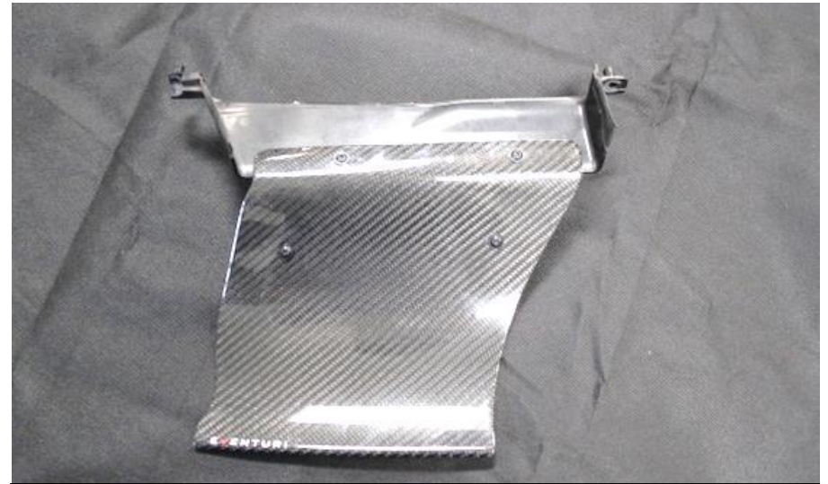
26. Locate the scoop as shown – secure with the supplied M5 black flange bolts and lock nuts – see next step.
