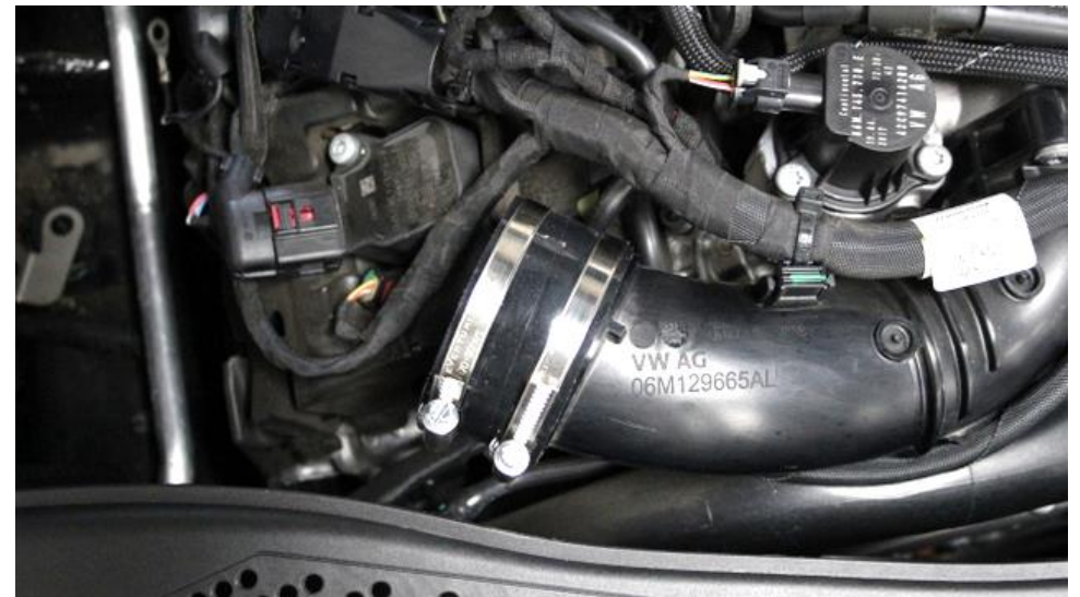
18. Push the supplied silicon coupler onto the turbo inlet tube and secure the hose clamp around the tube. Leave the other clamp loose.
