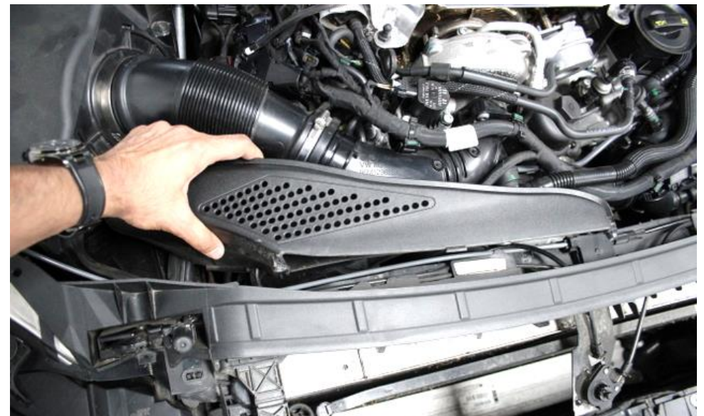
8. Remove the duct – it will already be loose after removing the 2 torx screws from step 4.
