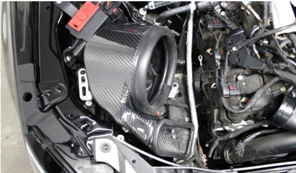
15. Locate the duct with the installed rubber mounts into place so that all 3 mounts push into the stock locations. It will help if you lightly lubricate the rubber mounts beforehand.
