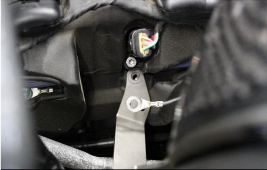
21. Rotate the housing so the bracket lines up with the threaded hole on the engine which had the Torx Screw removed in step 14.
