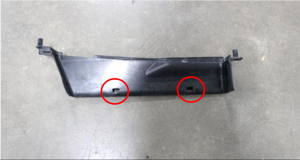
25. Take the front duct trim from step 5 – we will secure the carbon scoop to the circled holes.
