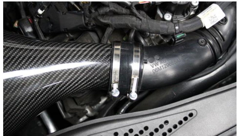
24. With the housing in place – secure the remaining hose clamp around the silicon coupler.
