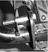
13) Connect the bottom of the shock to the lift bracket using a 10x55 hex bolt and 10mm lock nut.
