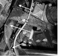
7) Disconnect it from the differential, cut the zip ties holding it in place, and pull it up through the hole near where the shock mounts to the frame.
