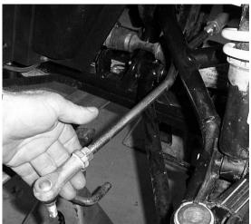
24) Make sure to reuse the washers, castle nut, and cotter pin to connect the end to the knuckle assembly but do not insert the cotter pin until you have checked the tow on the ATV so assemble both sides.
