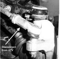
19) Remove just the rod and jam nut from the steering stem.
