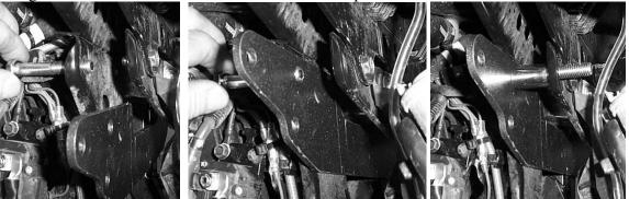
11) Place the front small spacer on the outside of the shock mount on the end of the bolt.
