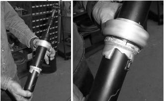
6) Place the stock spring(s) back onto the shock.
