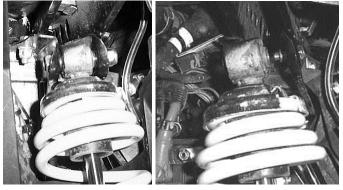
4) Using a spring compressor, compress the shock and remove the stock spring.
