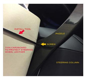
**Step 3:** In the reverse of Step 2, install the Carbonio carbon fiber paddle in the place of the original paddle. Again one screw will be easy to get to while the other will have very tight access. The following order works well:
