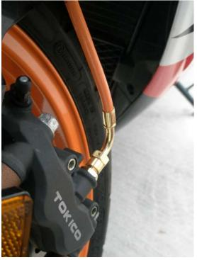
h. Left caliper, notice position of fitting
