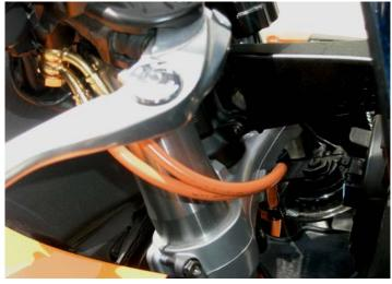
b. Routing from master cylinder to lower triple tree
