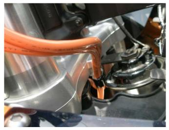
c. Routing at lower triple tree
