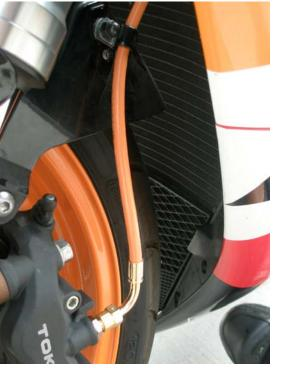
g. Right caliper, notice Galfer provided c-clip at fender
