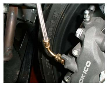
C. Right Caliper, notice the line is slightly away from the bike
