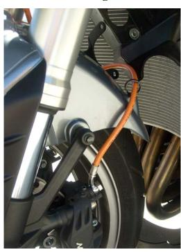
g. LINE C - Left caliper, notice OEM routing tabs
