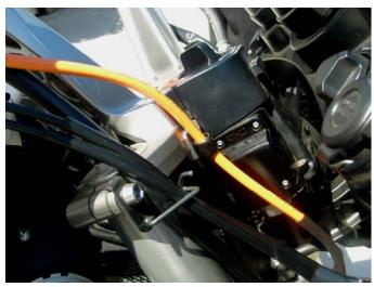
b. LINE A – Galfer c-clip at upper triple tree
