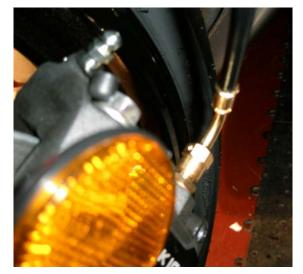
d. Left caliper, notice fitting is pointed away from the bike a bit
