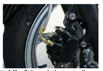
f. Hex fitting and adapter at caliper
