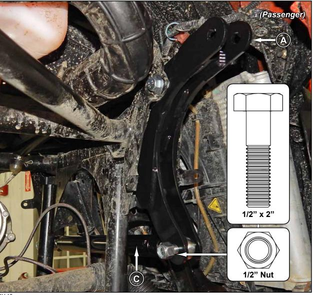
Tighten hardware completely.
